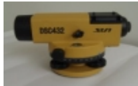
PLATE 2: Automatic level SUN DSC 432
