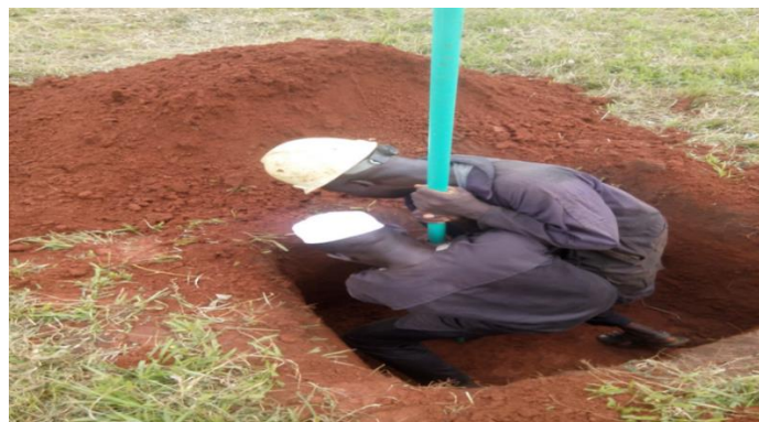
Plate 1b: Photograph showing the collections of undisturbed samples of 1.0m - 1.5m layer (Samples collection from the study areas of Irele)
