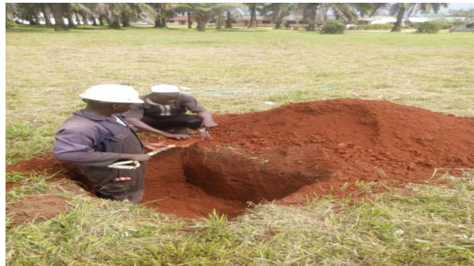
Plate 1a: Photograph of trial pit showing the collection of Samples from the study areas of Irele of disturbed samples of 1.0-2.5
