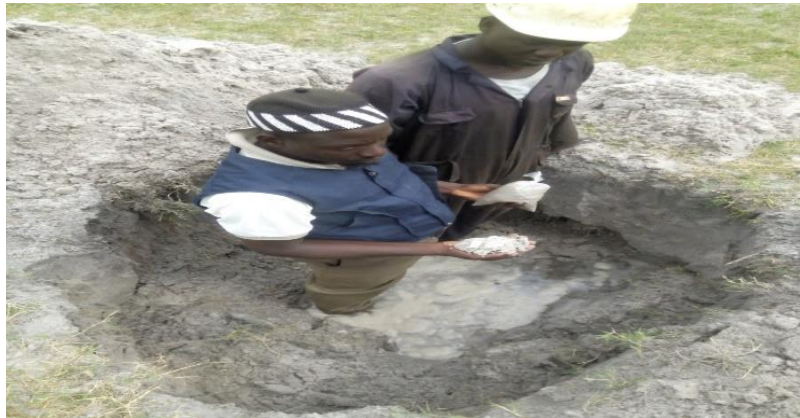
Plate 2a: Photograph of trial pit showing the collection disturbed samples of 0.5m- 2.5m Ilaje
