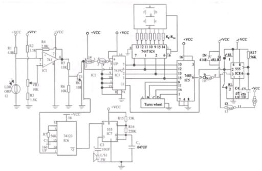
Figure 4: Complete Circuit Diagram of Automatic Control for a Bottling plant
