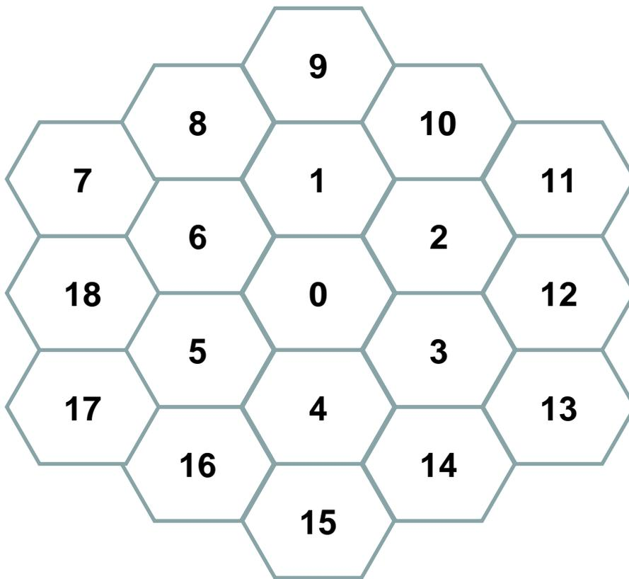
**Figure 4:** The cellular layout showing the two tiers of cells around cell 0
