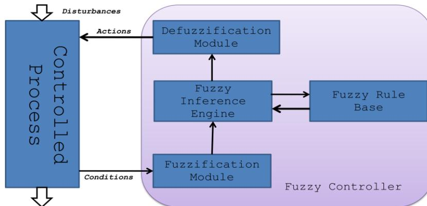
**Figure 2:** The components of a fuzzy controller processes
