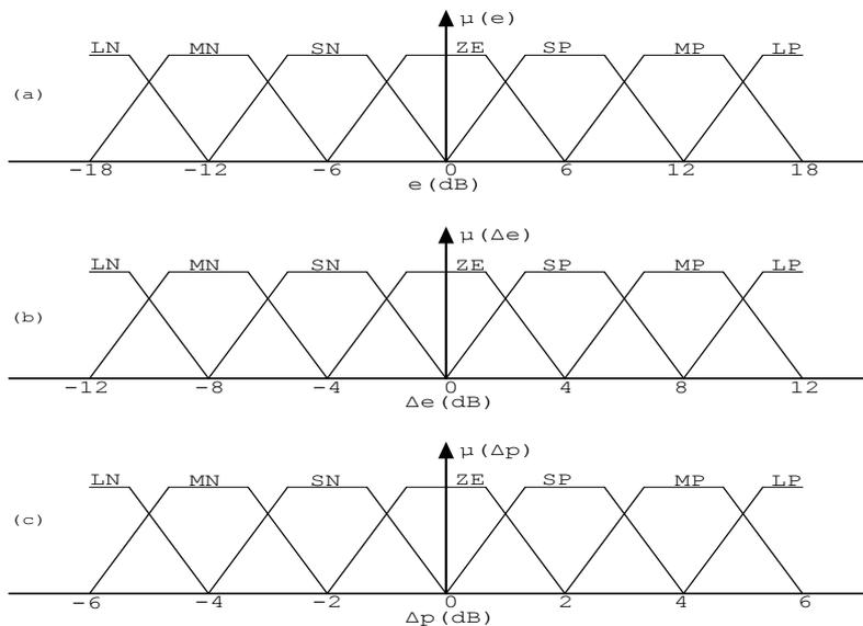
**Figure 3:** Graphical representation of the trapezoidal membership function for the fuzzy set values showing (a) the error (b) change in error (c) incremental power
