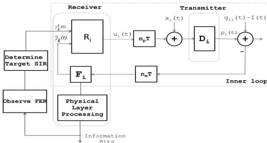
**Figure 1:** Closed loop power control schematic for SIR-Based Transmit Power Control showing inner and outer Control Loop process
