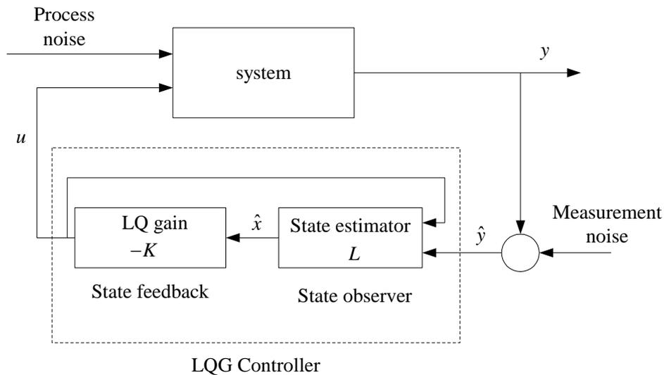
**Figure 2:** The schematic diagram of the closed-loop control system showing the LQG controller
