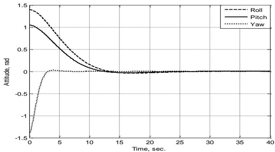
Figure 4(b): Simulation responses for LQG controller
