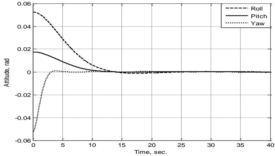
Figure 5(b): Simulation responses for LQG controller
