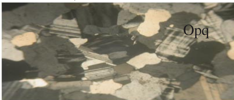
Cross polarization X 40 Pg-Plagioclase, Mi-Microcline, Qt-Quartz, Opq-Opaque mineral
