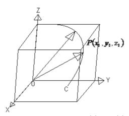
Let the parametric equation of curve C be x = f(u), y = g(u) and z = h(u), where f, g and h are continuously differentiable. If R = f(u)i + g(u)j + h(u)k, then a vector tangent to C at the point P is given thus:  $T_0 = \frac{dR}{du}|_{p}$ . In rectangular form this
