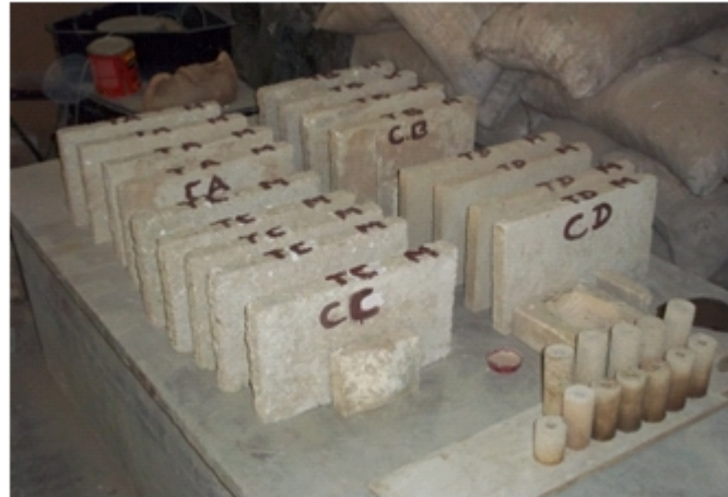
Fig. 8: Shelves Produced using Manual Ramming/Semi-Motorized Method
