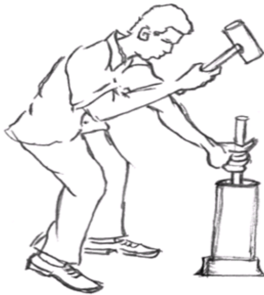
Figure 2: Manual ramming method used in Props Production Source: Studio Practice
