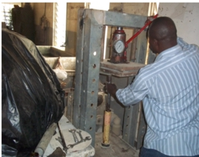
Fig. 7: The assembled machine/Pressing of Prop in Progress
