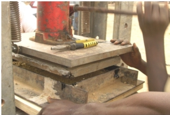
Fig. 6: Guiding for the proper fitting of the top metal plate into the angular frame containing shelf materials using semi-motorize mechanism
