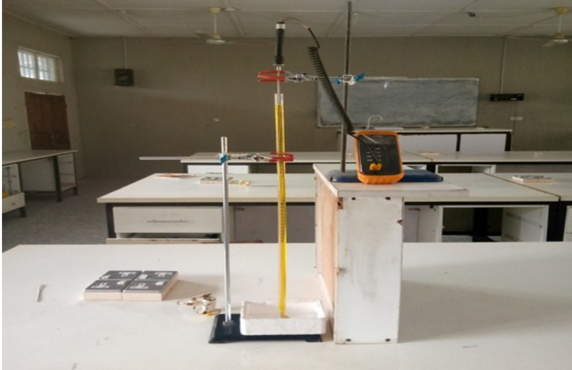
Figure 2: Experimental setup for the determination of viscosity
