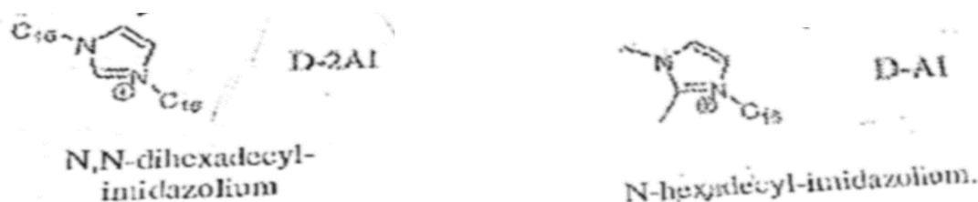
An N,N-dihexadecyl-imidazolium (D-2AI) modified clay was prepared and characterized as shown in the table below:
