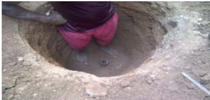
Figure 2: Trial pit with soil core cutter Source: Fieldwork, 2015
